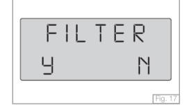
Where "Y" (Yes) will be flashing. To select "N" (No) press one of the 2 arrow keys "N" will start to flash. If you press the button "x", the control of the softener filter remains deactivated, quitting the programming function and returning to the initial screen.
